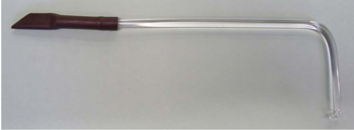
Figure 9. Picture of a rubber policeman attached to a glass hockey stick.
